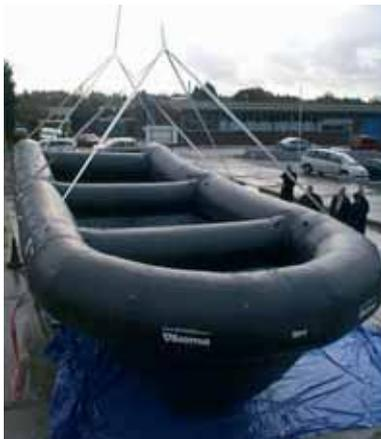
Inflatable Oil Storage Barges can be used to transport oil products in port and marine operations or for the intermediate storage/transportation of recovered oil. Alternatively, they can also be used for the transportation of all kinds of low-density products.
